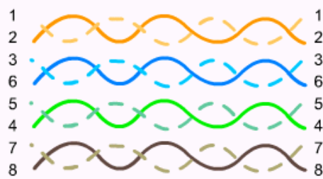
Correct T568B Wiring
